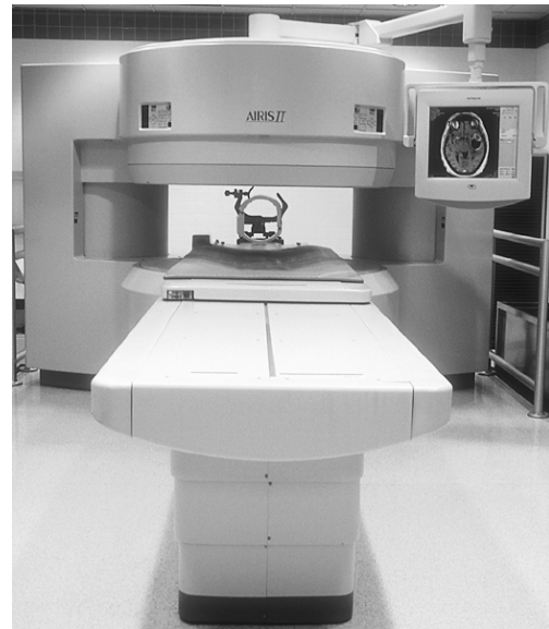
Figure 5: Viewed from the front, this open MRI resembles a bagel more than a donut, allowing the person being scanned more room.
